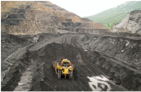
RCT has commissioned ControlMaster® Teleremote technology on this CAT D11T dozer at Teck Resources Coal Mountain Operations in Canada.
