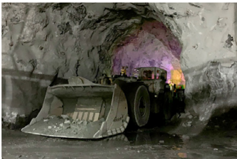
RCT has commissioned ControlMaster® Guidance Automation onto multiple machines including this CAT 2900 underground loader for MATSA Resources in Spain.
