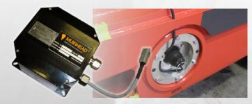
Safeguard operators during refuelling to prevent incidents such as driving off with the fuel nozzle still attached by ensuring the machine remains locked out, in a safe state for the duration of the daily task.
